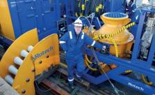
**Rotech Subsea Ltd** were contracted to Hughes Sub Surface Engineering to carry out Export Cable Deburial operations. A fault was reported on the 132kV export circuit 2 of the OFTO and was located (by TDR tests) at 8.17km from the West offshore platform; at this location the cable is buried to a depth of 1.5m and the water depth is 5m LAT.
